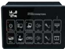
The touchpad consists of 15 touch keys, each key with LED backlight
